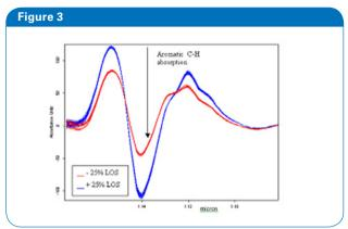
FT-NIR derivative spectra spectra (1.18 - 1.09 micron) of two tablet samples with +/- 25% deviation from the target concentration.
