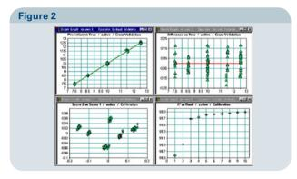
Cross validation results of PLS based models for the prediction active drug in a tablet ( $R^2$ =99.72, RMSECV=0.09mg/tablet).
