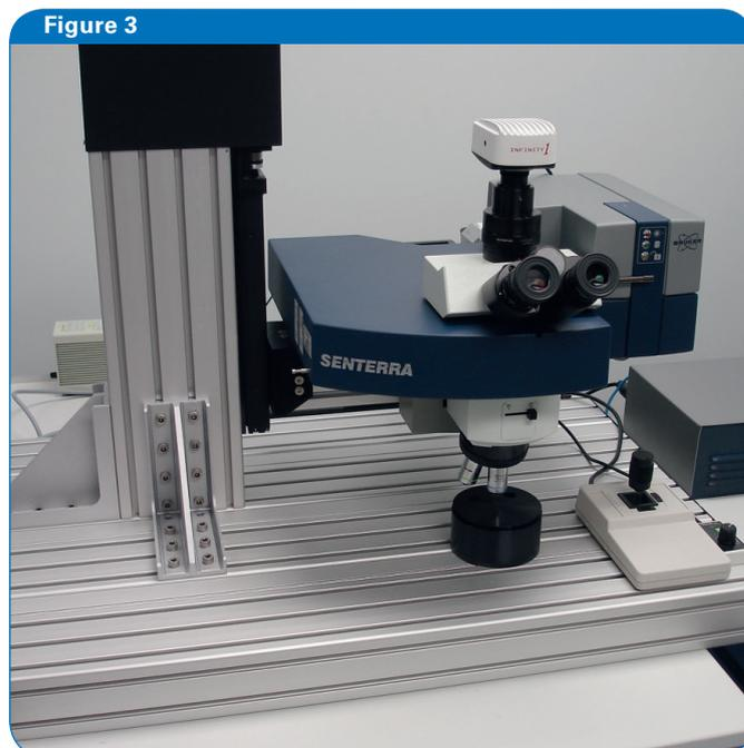
SENTERRA Raman microscope mounted on a z-stage.
