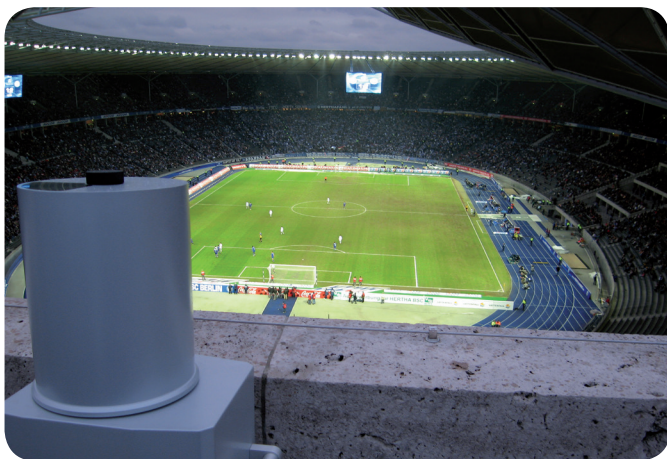
Figure 2. Monitoring of the air in the Olympic stadium in Berlin using SIGIS 2.
