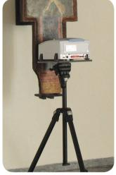
Figure 8: The ALPHA FT-IR spectrometer with the tripod option at "Pinacoteca Nazionale di Bologna" during material screening.
