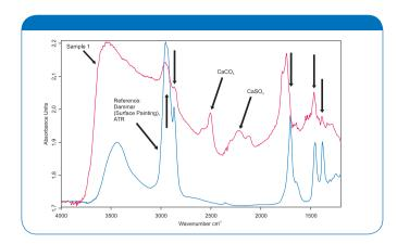
Figure 4: Spectrum of an area of the mural painting before cleaning showing typical absorbance of a terpenic varnish, calcium carbonate CaCO<sub>2</sub> and calcium sulfate CaSO<sub>4</sub>.
