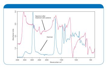
Figure 5: Spectrum (red) of the mural painting after treatment with acetone. The typical absorption bands of terpenic varnish (blue) are missing showing a successful treatment of the mural painting.
