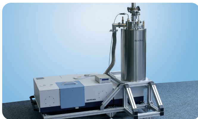
Fig. 8: Customized module for Silicon impurity photoluminescence, adapted to a VERTEX80v FTIR spectrometer. The samples are mounted in a liquid Helium bath cryostat in order to compensate the heat, created by the visible excitation laser
