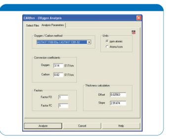
Fig. 1: Screenshot of the OPUS/SEMI software package for the comfortable determination of Carbon and Oxygen content.
