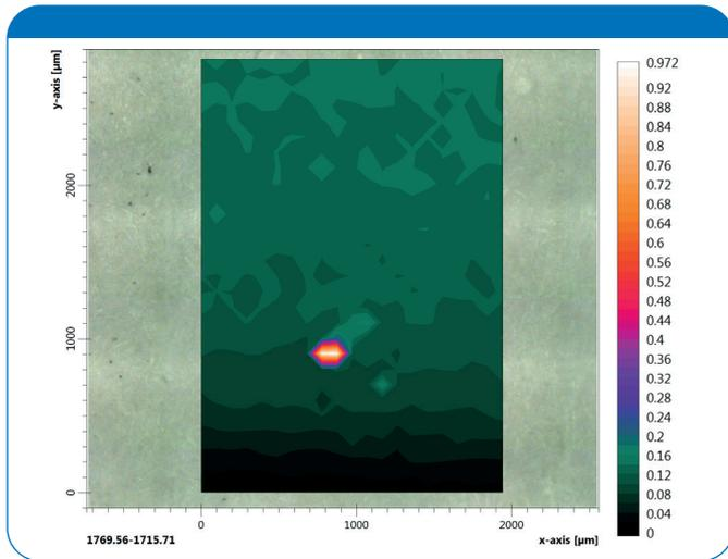
Figure 7: Chemical image of the punctual defect.
