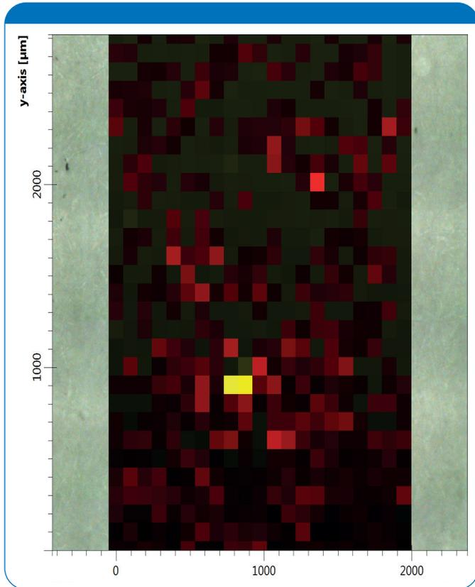
Figure 8: WTA-image that shows the distribution of the filler calcium carbonate (red) and the point defect (yellow).
