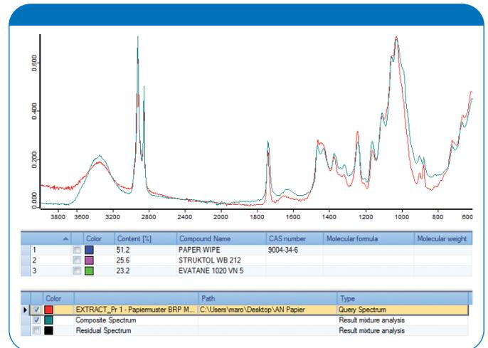
Figure 6: Result of the mixture analysis of the punctual defect. The composite spectrum calculated from the single component spectra (turquoise) almost perfectly matches the sample spectrum (red).
