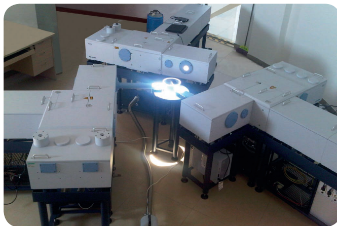
Fig. 2: Arrangement of three compact IFS 125HR spectrometers installed in the new astronomical observatory at the Shenzhen Meteorological Bureau in China.
