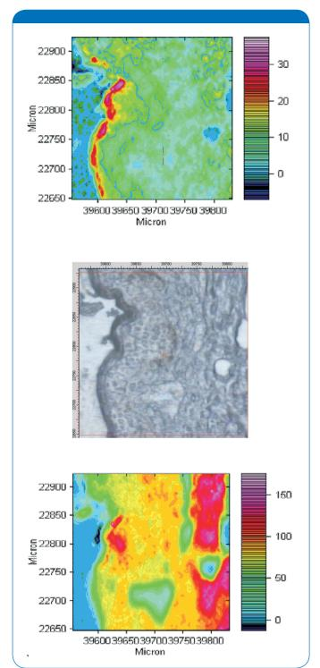
Fig. 1: IR imaging of human skin tissue. Middle panel: transverse section  $(250 \times 250 \mu m; 15 \mu m)$ , was measured using a Bruker HYPE-RION (8cm-1 resolution, 15x, transmission). Upper panel: integrated signal intensity in the CH stretch vibration range (3000 - 2800 cm-1) = lipid distribution. Lower panel: integrated signal intensity in amide range (1720 - 1480 cm-1) = protein distribution.
