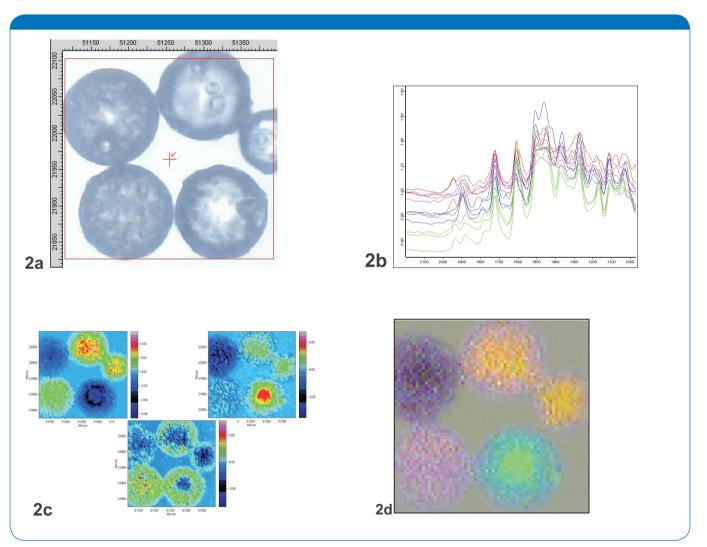
Fig. 2: IR image of polystyrene beads (8cm<sup>-1</sup> resolution, 15x, transmission): Beads lock very similar in the visible image (2a). 2b: Representative IR spectra for a number of detector pixels. 2c: Similarity of the original spectra to the three relevant principal components; 2d: RGB image made up of the three relevant principal components.
